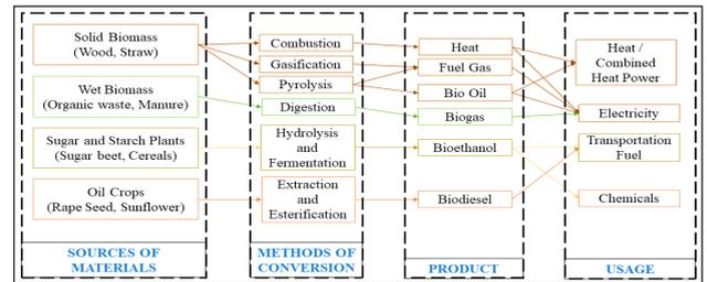
Fig. 4: Schematic pathway of power generation
