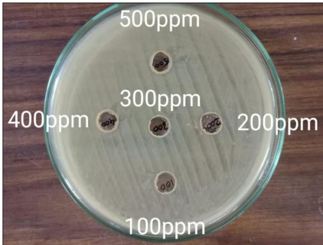
**Fig. 2:** Sodium hypochlorite at 100 ppm (0.01%), 200 ppm (0.02%), 300 ppm (0.03%), 400 ppm (0.04%), 500 ppm (0.05%) where no inhibition zones were found
