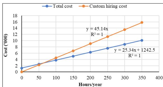
**Fig. 1:** Breakeven point representation for manual drawn rotor weeder
