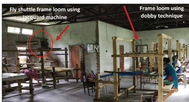
Fig 3: Handloom unit with different types of handlooms and weaving process
