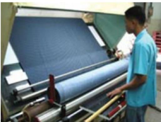
Fig. 2: Modern manual fabric inspection table.
