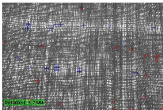
Fig. 8: Real time defect detect and total defect in percentage
