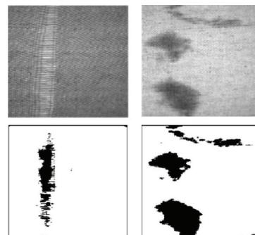
Fig. 7: Defect area segmentation using image processing
