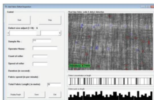
Fig. 9: Software for real time defect detect, defect % and display graph of moving fabric on inspection table
