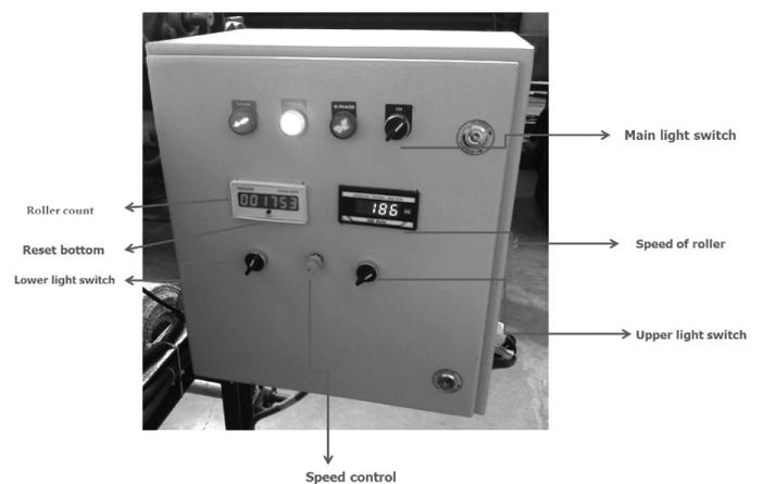
Fig. 5: Control panel of inspection table
